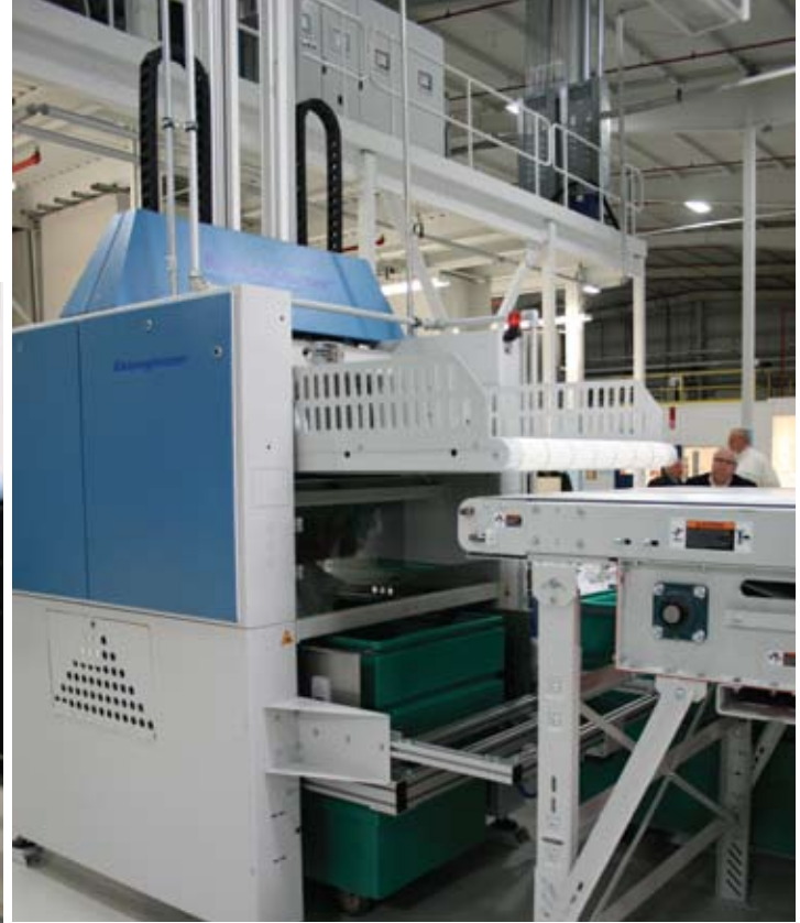
This sheet picker, or linen separator, breaks up tangled clumps of sheets to make it easier for employees to feed them into the ironer.
