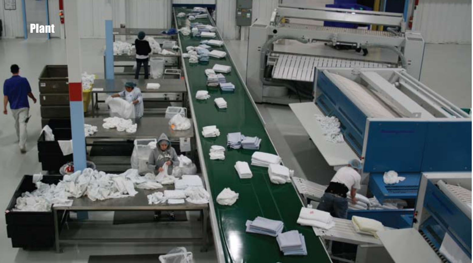
Employees at left hand fold linens and place stacks onto a conveyor belt that moves them to packout. On the right side, goods emerge from ironers and folding/stacking equipment. Employees place these goods on the conveyor as well.
