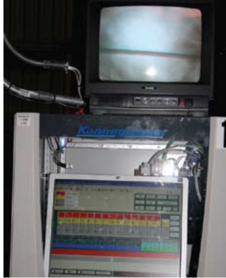
At left, an employee places finished, folded goods on a cart. Above, a monitor screen tracks goods in one of the plant's two tunnel washers, each of which has 14, 165 lb. compartments.
