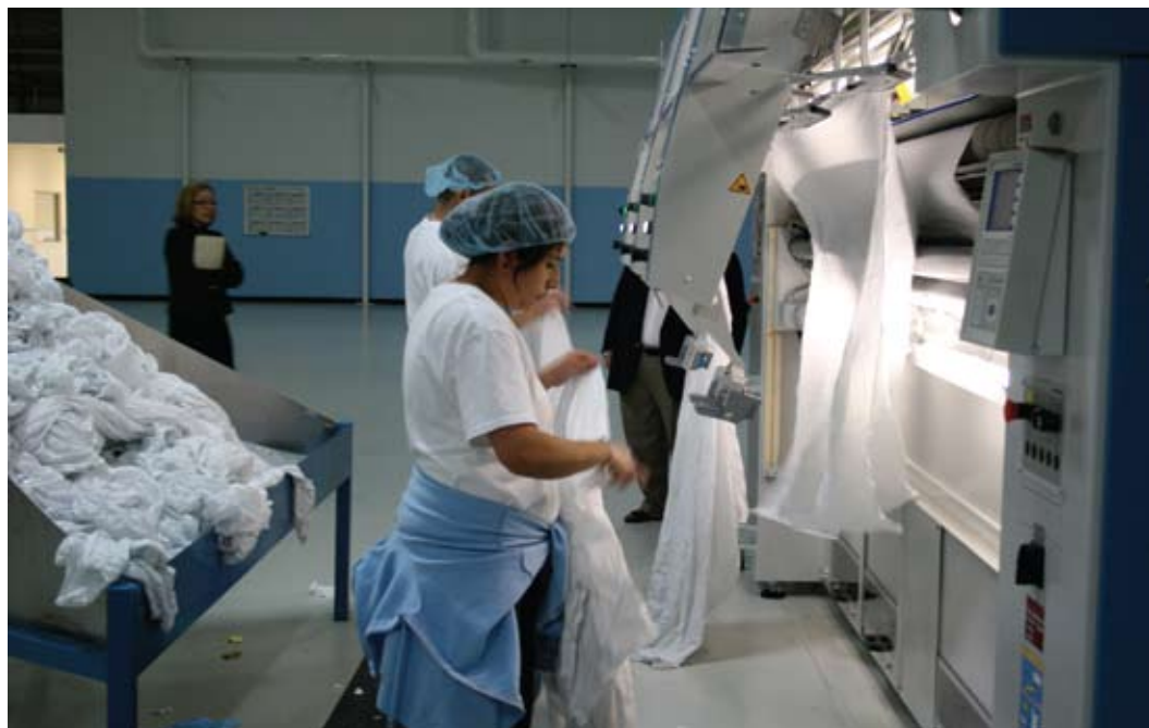
Employees feed separated sheets into the spreader/feeder before entering the ironer. Company President Judy Reino stands at left.
