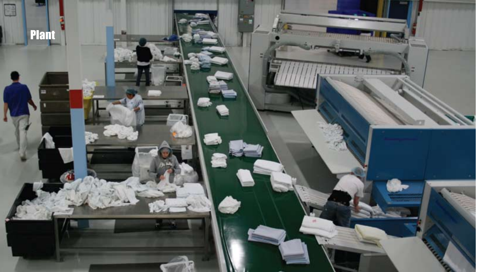
Employees at left hand fold linens and place stacks onto a conveyor belt that moves them to packout. On the right side, goods emerge from ironers and folding/stacking equipment. Employees place these goods on the conveyor as well.
