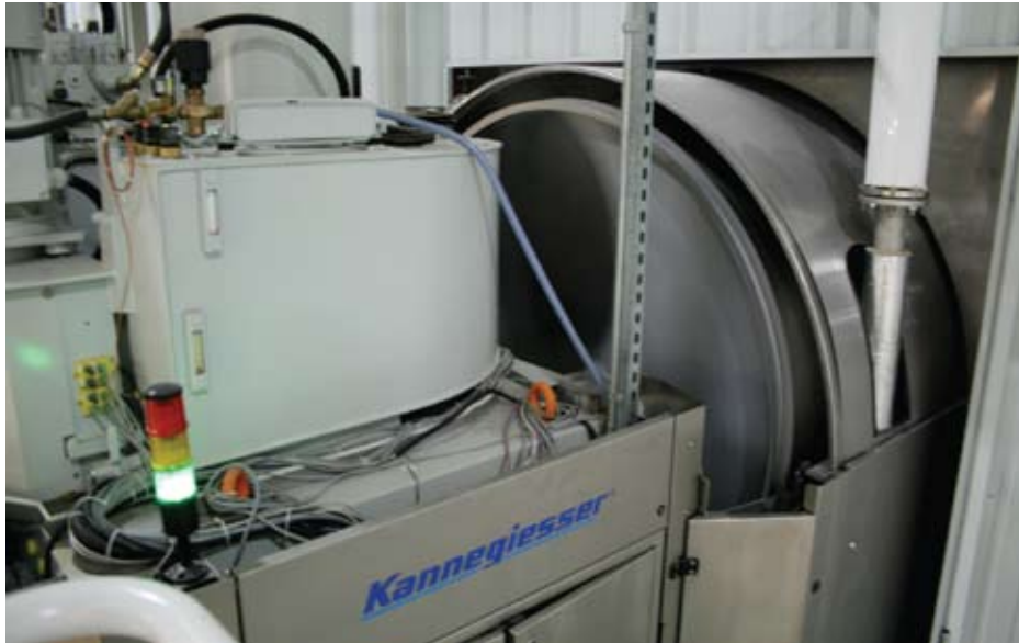
A clean-side view of the discharge end of the tunnel and press, where cakes of clean goods will emerge for movement to the finishing department or the dryers.
