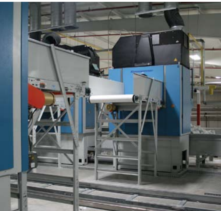
Cakes of clean wet goods move on the conveyor at left and then onto the platform for movement into the dryer.
